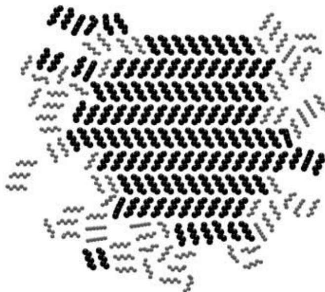
Figure 2. Top view of the time averaged configuration of the first adsorbed layer of n -hexane multilayer on graphite. Molecules in black have at least one intermolecular distance that is less than 5.0 Å. Hydrogen atoms are not shown for clarity.
